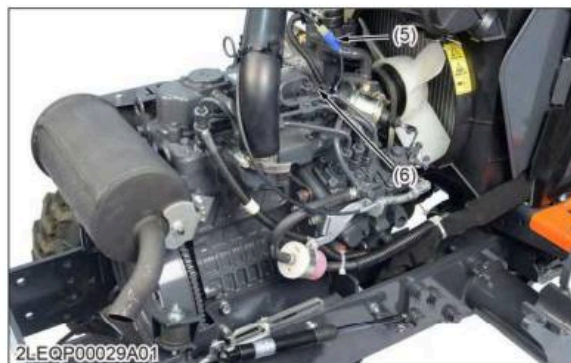
(5) Stop solenoid (6) Glow plug
