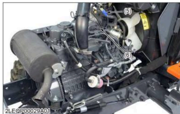
(5) Stop solenoid (6) Glow plug
