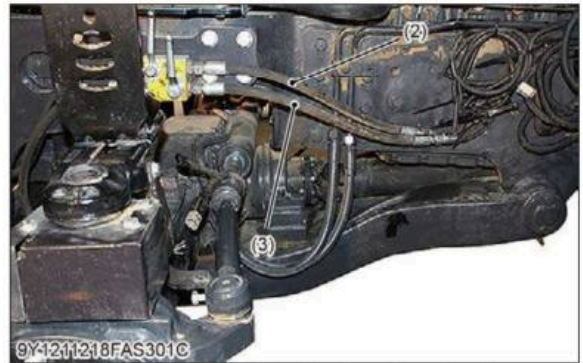
(1) Front 3-point hitch lock shift box (2) Front 3-point hitch hose 1 (3) Front 3-point hitch hose 2
