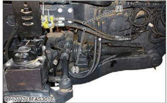
(1) Front 3-point hitch lock shift box (2) Front 3-point hitch hose 1 (3) Front 3-point hitch hose 2
