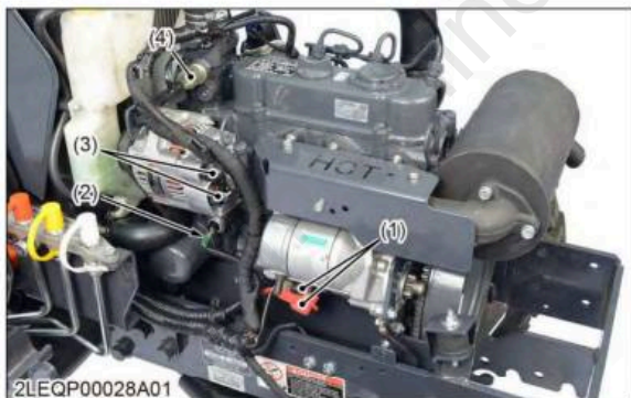
(1) Starter connectors (4) Coolant temperature switch (2) Oil pressure switch (3) Alternator connectors
