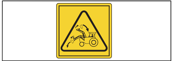
Fig. 38 Keep your eye on the implement, objects may fall backwards onto the operator.
