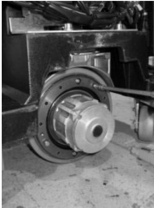
Figure 6.2. Removing the drive wheel fixing screws on 1,300 and 1,600 kg capacity trucks
