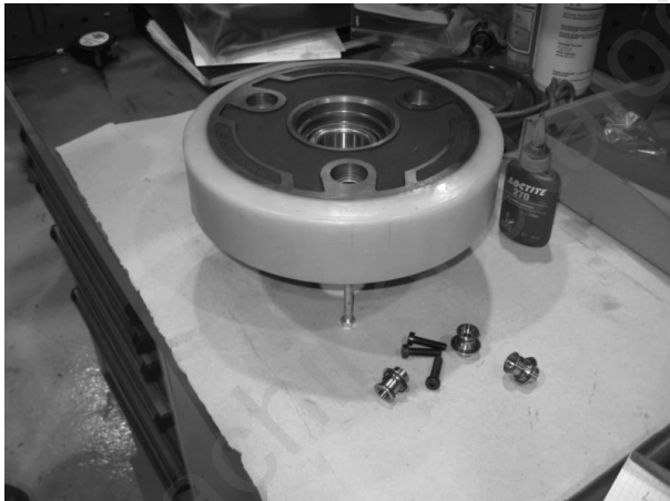
Figure: 6.6 Wheel position over brake ring
