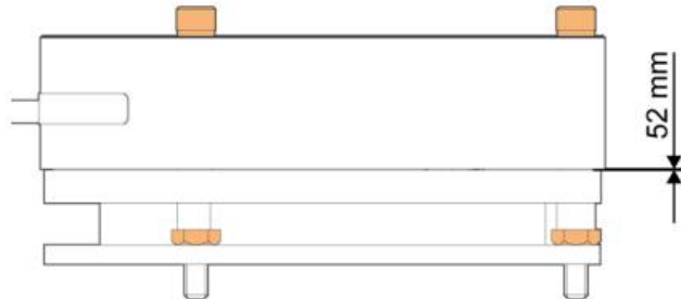
Figure 114. Adjusting the air gap of the magnetic brake
