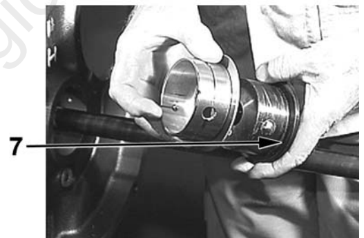
7 internal squeeze head for bearing bushes 5 and 6 (tool no. 84.7)
