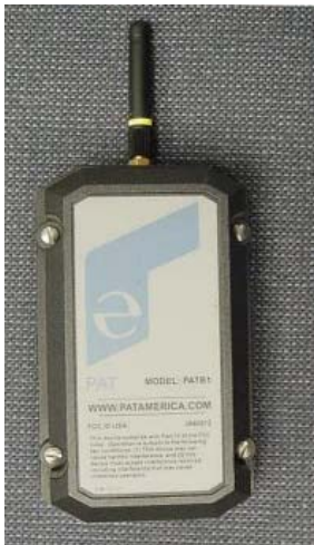
Radio A2B transmitter with antenna 031-300-060-487 Antenna only 031-300-050-579
